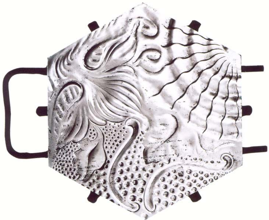
La casa Escofet conserva el molde metálico original del mosaico de Gaudí The Escofet company still has the original metal mould for tiles designed by Gaudí
